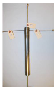
Construct pilot-scale (2 lb/day H 2 ) Separators & DOE test protocol durability tests
