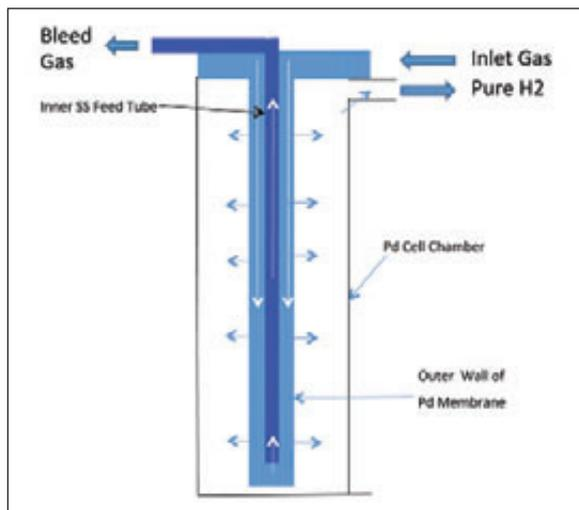
Figure 3: Power and Energy's inside-out micro-channel palladium purifier with vacuum brazing and laser weld improves durability over previous designs using traditional welding techniques. The welding of palladium to stainless steel will weaken the joint when performed with traditional weld methods. Using laser welding improves repeatability and long-term durability
