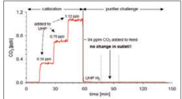
Figure 2: A palladium purifier is challenged with up to 94 ppm of CO<sub>2</sub> with no change in outlet purity. Outlet purity is below 50 ppt
