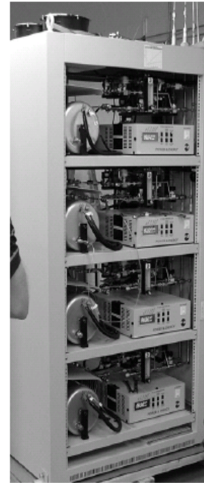
High Capacity 1300 slpm Modular H 2 Purifier System
